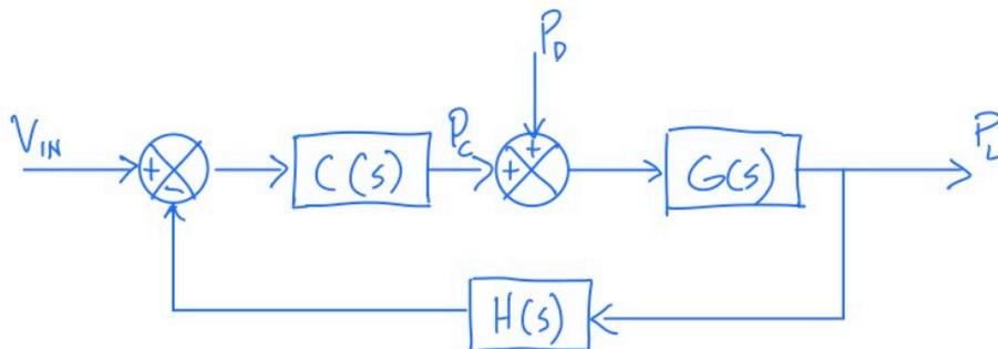
where  $C(s)$  is the controller,  $G(s)$  is the plant (the thermal characteristics of the infant), and  $H(s) = 1$  is a sensor in the feedback loop. Assume that
